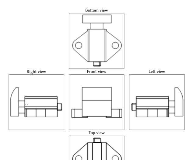
Spring Stop Buttons – Flat Face (Type C), Standard Force, Steel Plunger
