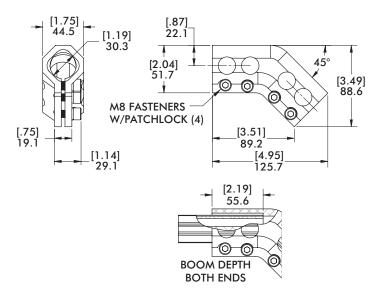
Specifications: Max. Static Clamp Load: 271Nm [200 ft-lb]
